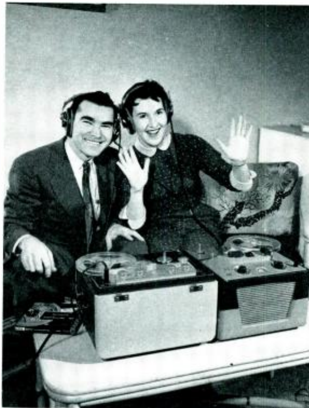
The results are worth the effort! Binaural recording brings a sound realism that must be heard to be appreciated. One earphone from each headset is interchanged so each ear hears a separate channel.
